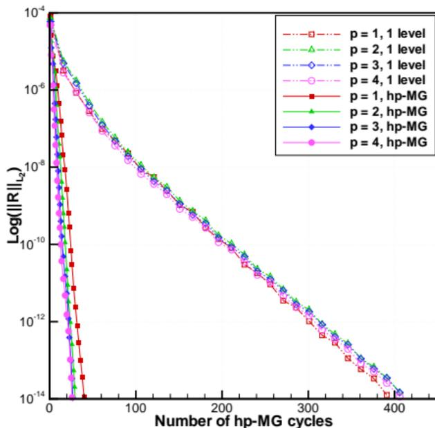
$L_2$ -norm of residual vs. MG cycles
