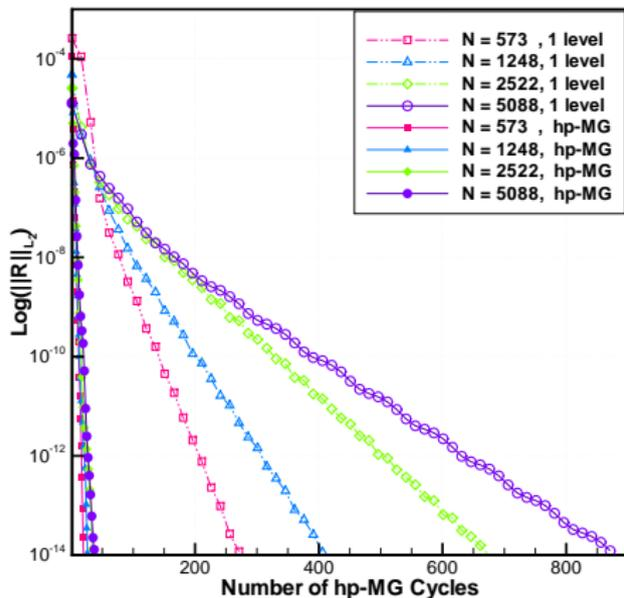
$L_2$ -norm of residual vs. MG cycles
