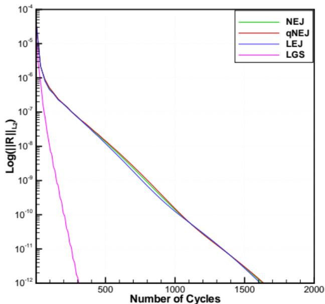
$L_2$ -norm of residual vs. MG cycles
