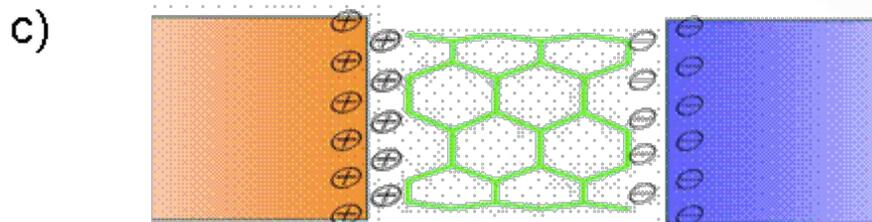
(a) Electrostatic potential energy distribution along the central axis at  $t = 0.02$ , 1 and 12 fs. (b) Charge distribution along Al-CNT-Al at  $t = 4$  fs. (c) Schematic diagram showing induced charge accumulation at two interfaces which forms an effective capacitor.
