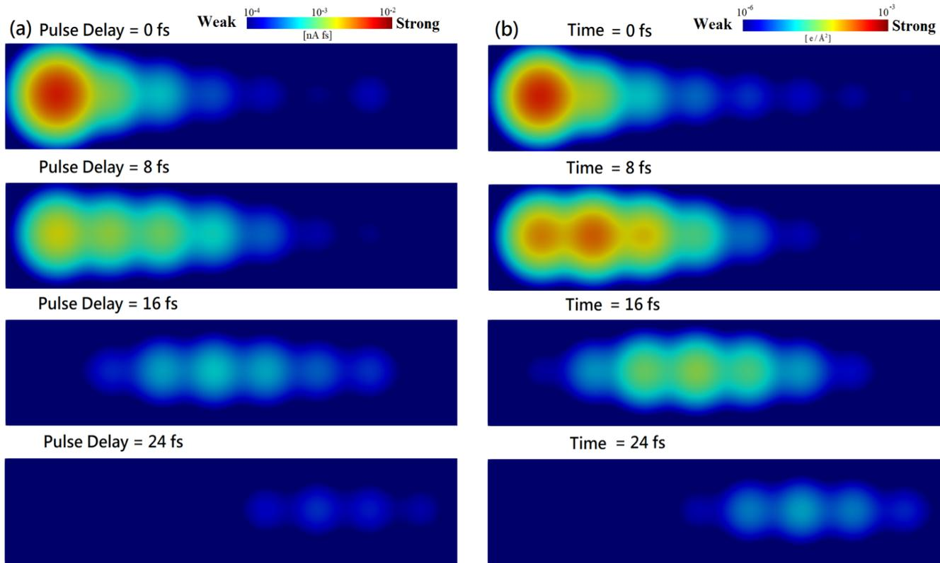
Left panel: pump-probe STM images with various pulse delays As indicated. Color reflects the magnitude of integrated current on a log scale (projected on real space). Right panel: electron density images (obtained by projecting occupation of LUMOs on real space) at the same times. Color reflects the magnitude of electron density on a log scale.
